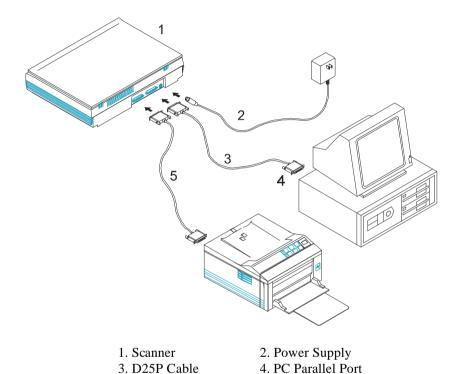
Figure 2-2 AV363C scanner cable connection
